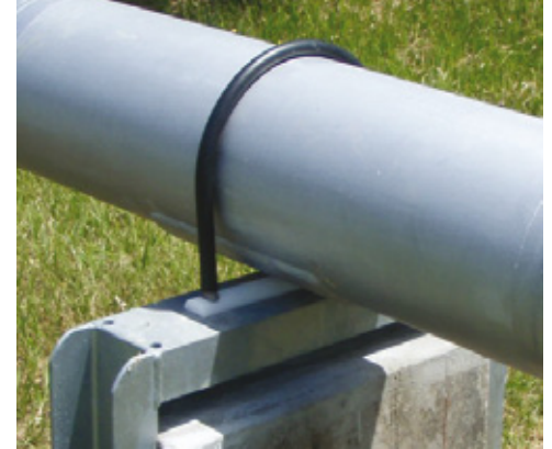
I-Rod® eliminates the crevice by minimizing the contact area and allowing any moisture to evaporate. It's also much easier to inspect.
